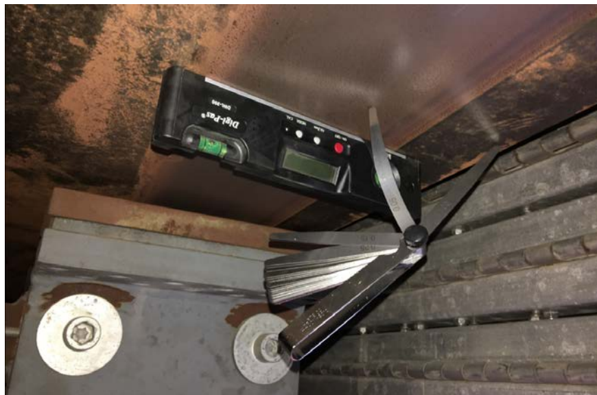
Magellan Track Plate Wear Measurement with Feeler Gauge
