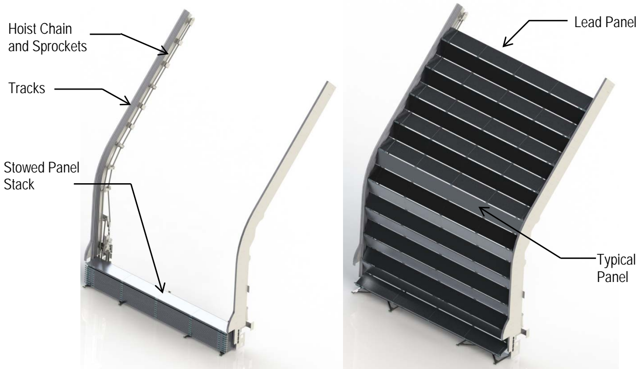
Windscreen – Stowed (Left) and Deployed (Right)
