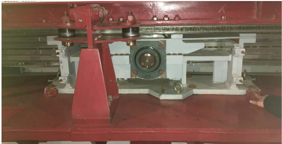
Idler Bogie Assembly - Magellan
