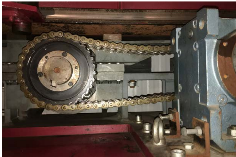
Drive Bogie Assembly - Magellan
