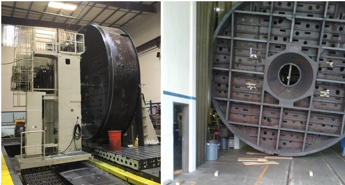
Figure 5. These photos show the M1 cell in the shop during its fabrication. left panel: The front surface of the top plate is visible. right panel: In this view of the rear side of the cell, the cone that will interface to the Cassegrain instrument derotator is visible.
