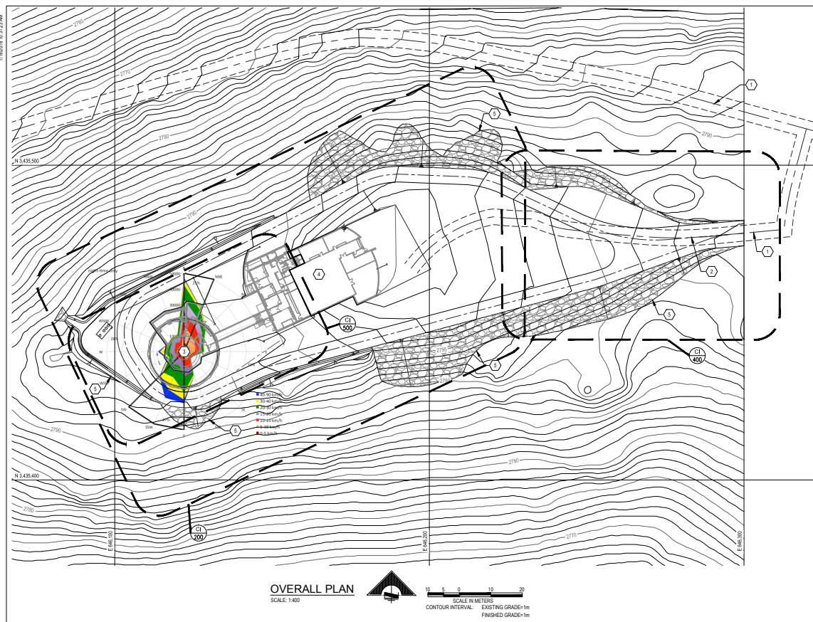
Figure 9: The proposed TSPM facility design and wind rose are overlaid on a topographic map of the site. The telescope enclosure is “downslope” and close to “cross-wind” from the support building (Figure 2). The terrain modifications will place ground level for the telescope pier at 2794 m above sea level and the far end of the support building at 2800.5m above sea level. The ground level for the pier is above the surrounding terrain in all directions, except towards the north, where it is 1 m lower, and for the directions where the wind will blow over the support building. In this last case, which occurs 17.5% of the time, the roof of the support building is approximately at the level of the elevation axis.
