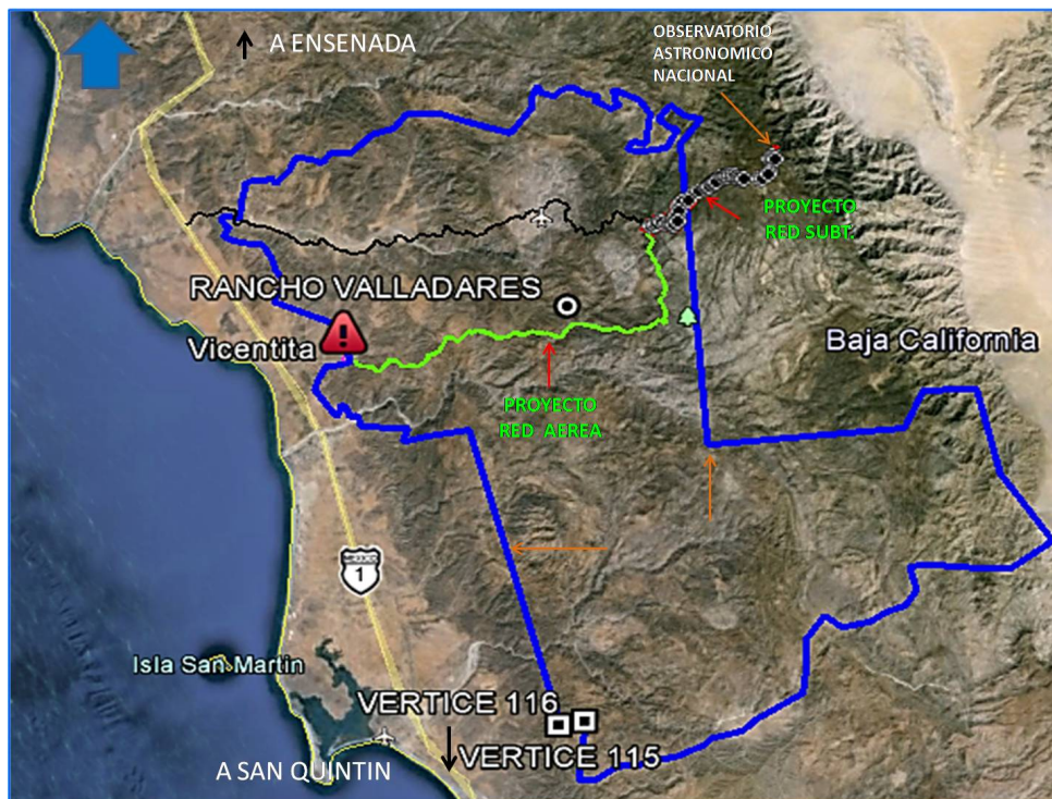
Figure 15: This map shows the path of the electricity line that will connect the OAN-SPM to the national electricity grid. The part shown in green will be an aerial line that will branch from an existing power line. The part shown with black diamonds will be a buried line and follows the south side of the road to the OAN-SPM, shown as the black line that connects to the transpeninsular highway (“MEXICO 1”, yellow line). (Do not be fooled by the airplane symbol. It corresponds to a very, very rudimentary airstrip!)
