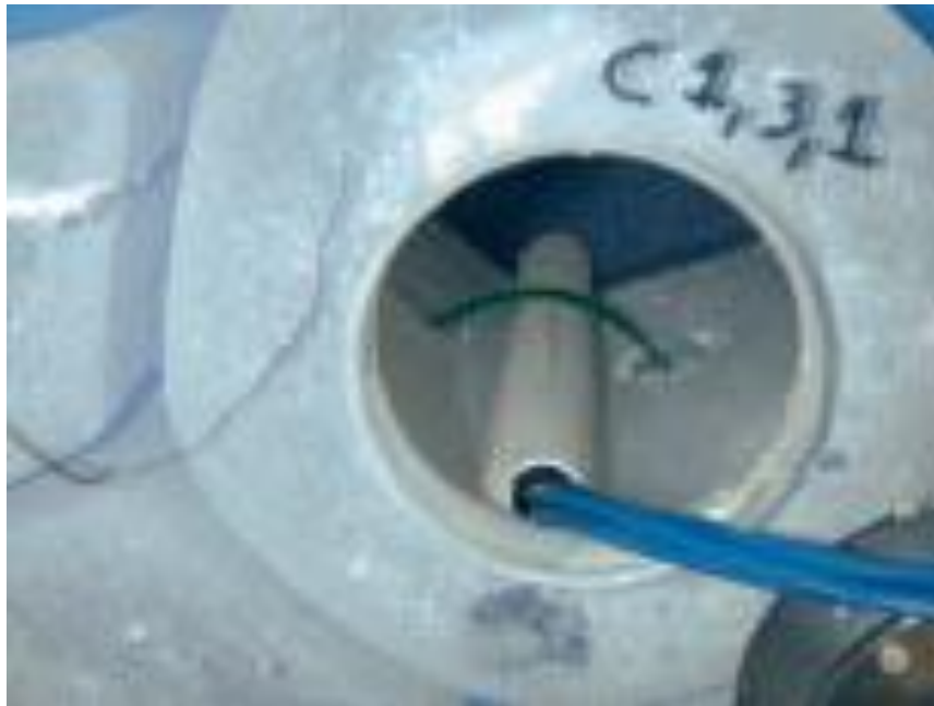
Figure 5-40 Thermocouple installation example
